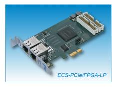
EtherCAT Slave Interface for PCI Express The ECS-PCIe/FPGA is an EtherCAT Slave Controller board designed for the PCI Express bus. It utilizes a Beckhoff IP-core which is implemented in an Altera® FPGA and configured for 8 FMMUs, 8 Sync Managers, 60 kB DPRAM and 64 bit
