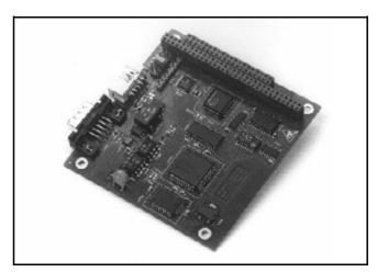
Like all low cost CAN boards there are restrictions in comfort and data reliability with the CAN-PC104/200 due to the simple design of these boards. A reception without data loss can not be guaranteed in these designs, because it depends on the bitrate, the performance and the operating system of the host CPU.
