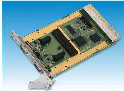
The CPCI-CAN/400-2 provides high resolution hardware timestamps.
