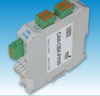
Simple resistance measurements can also be performed. Pt- and Ni-resistance sensors are supported. The sensor resistors can be connected in two- or four-wire configuration. The conversion of the four sensor resistor inputs is realized by four independent  $\Sigma\Delta$ -converters.
